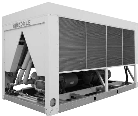
Figure 13.7 Air-cooled water chiller, nominal 600 kW capacity with two R134a refrigerant circuits, single shell and tube evaporator, and capacity controlled semi-hermetic screw compressors (Airedale)
