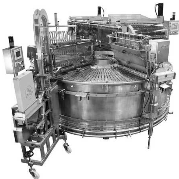
Figure 16.7 Novelty ice-cream stick product machine (Gram)
