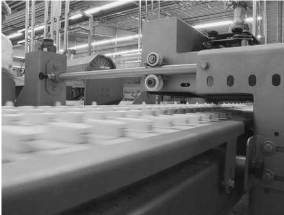
Figure 16.6 Stickline for ice-cream products (Gram)
