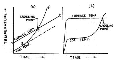
**1) Ignition temperature:** The ignition temperature of the coal decreases with increasing oxidation of coal.
